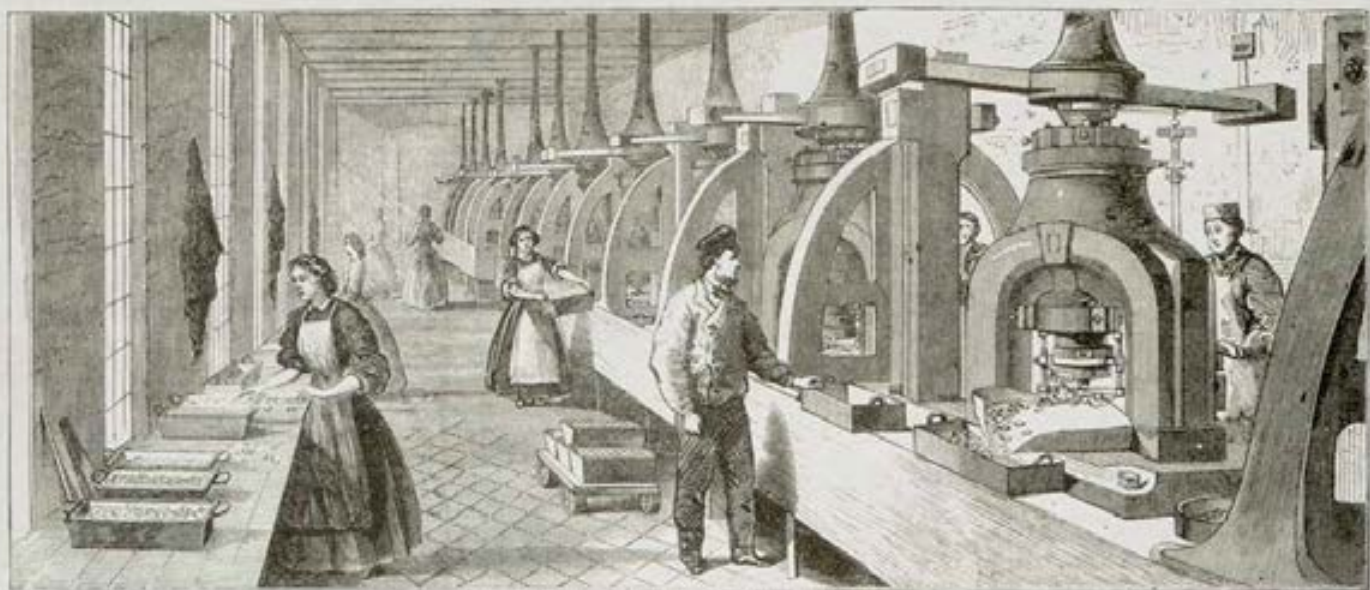
THE COINING-PRISSES, MEMRS. RALPH HEATON AND SONS' MINT.
